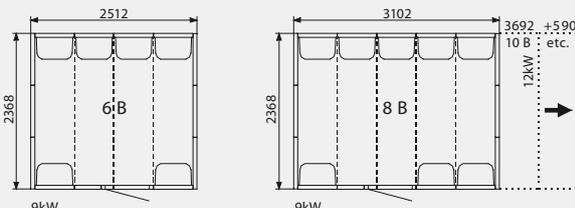
Glass wall sections and service walls are available in the widths 398, 588 and 778 mm. They can replace corresponding sections in Elysée rooms at no additional charge.
