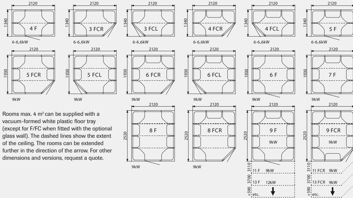
Rooms max. 4 m<sup>2</sup> can be supplied with a vacuum-formed white plastic floor tray (except for F/FC when fitted with the optional glass wall). The dashed lines show the extent of the ceiling. The rooms can be extended further in the direction of the arrow. For other dimensions and versions, request a quote.
