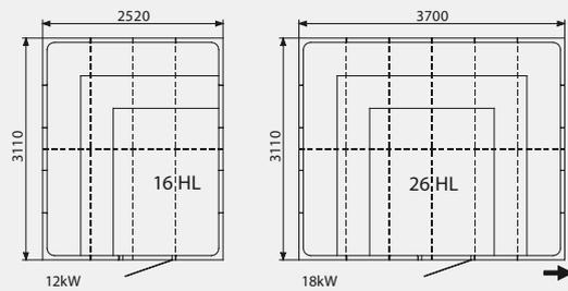
The dashed lines show the extent of the ceiling. The rooms can be extended further in the direction of the arrow. For other dimensions and versions, request a quote. Glass wall sections and service walls are available in the widths 398, 588 and 778 mm. They can replace corresponding sections in Excellent rooms at no extra charge.
