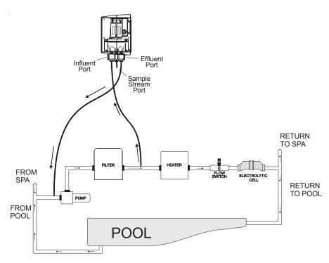
Drill and tap a 1/4" NPT hole using a 7/16" drill bit on the return side of the pool plumbing at a location just downstream of the filter, but upstream from the AQL-CL Electrolytic Cell. Use caution not to tap tapered threads too deeply. Using teflon plumber's tape, install a tubing connector into the hole. Run flex tubing from the tubing connector to the influent Probe Cell port. Push the flex tubing all the way into the pressure fitting to seat.
