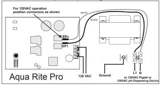
**IMPORTANT:** The dispensing device must be powered by the same voltage used to power the Aqua Rite Pro. Configure the output voltage to the pH device by moving the wiring connections on the mainboard according to the diagrams on page 7.
