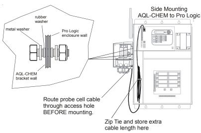
**Remote surface mounting the AQL-CHEM:** The Probe Cell can be mounted up to 15' away from the Aqua Rite Pro or the Pro Logic (limited by length of cable). Use the four mounting holes on the back of the bracket when surfacing mounting. Common wood screws can be used for most applications.
